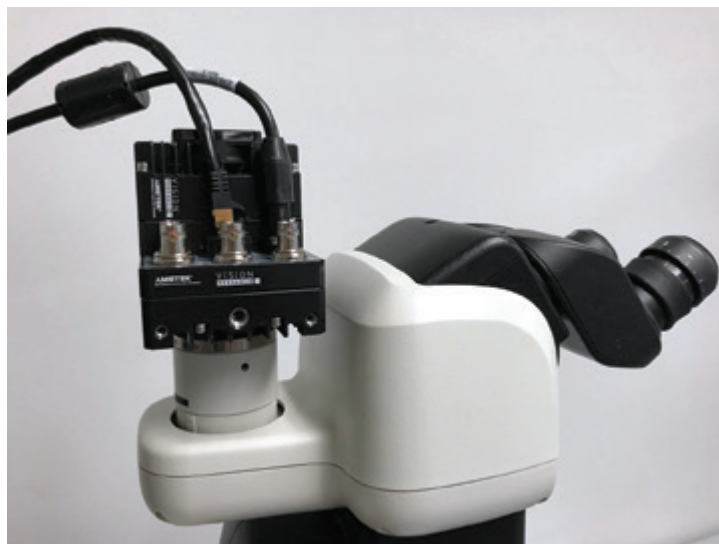
Miro C110 (connector view) mounted on a microscope
